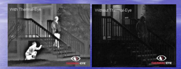
Thermal imagers measure heat, which is in the infrared portion of the spectrum
